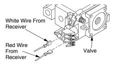
Figure 20 - Connecting Wires
